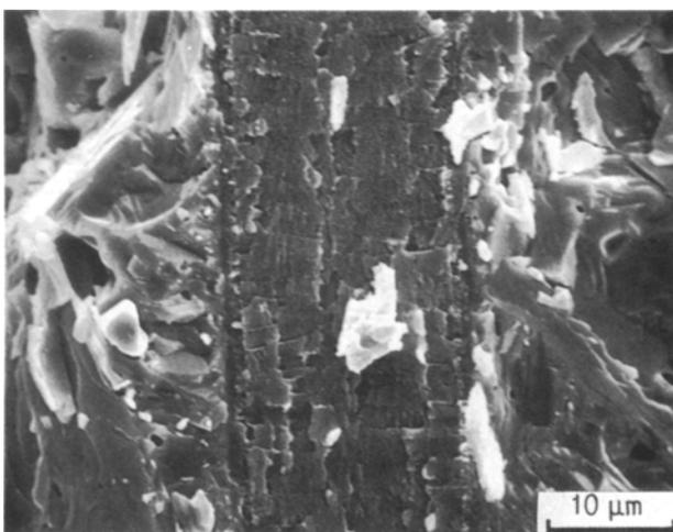
Figure 3 Fractograph of a composite sample heated to 400 °C for 90 min.
